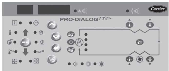
PRO-DIALOG Plus operator interface
